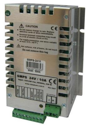
The units provide a "boost charge" input as a standard feature. When this input is pulled to battery negative, the output voltage of the charger will be set to the boost charge voltage. This feature may be used temporarily to improve battery life.
